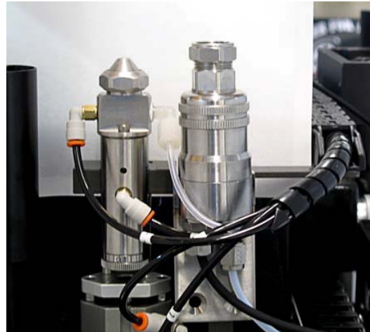
A.C.E. New Drop-Jet fluxer nozzle (Right) and standard nozzle (Left)
